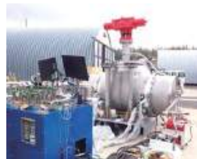
Prototype for LH 2 tests at JAXA Noshiro Rocket Testing Center (800A, 32" )
