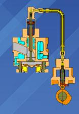
The LA series uses fuel-efficient marine engines with consideration for low NOx emission (reduction of CO2). The LA series reduces noise and prevents oil splashing by adopting a hydraulic valve driving system. By equipping an L-save ring on the upper part of the cylinder liner, surface wear of the cylinder liner is lessened and lubricating oil consumption is reduced.
