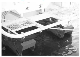
Ishigaki Co. Ltd., a leading Japanese manufacturer of water jet propellers, delivered them in December 2008 for installation in a high-speed patrol craft of the Japanese Coast Guard. The vessel, delivered to the JCG in March 2008, is now in operation.
