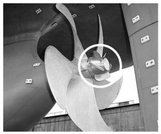
PBCF bolster the propeller's propulsion efficiency
