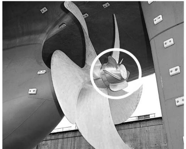
PBCF bolster the propeller's propulsion efficiency
