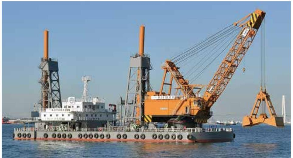
GE Series (All Electric Crane with Hybrid System)
