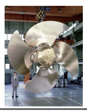
As the torque-rich of main engine caused by the fouling of the hull or the effect of waves and wind can be avoidable by adjusting CPP pitch angle and speed properly through ALC or combination control, when building the vessel, the main engine output can be minimized compared with FPP without considering margin to reduce fuel consumption.
