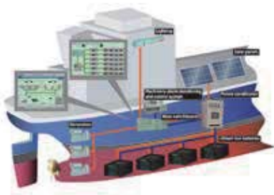
Fig.2 Li-ion Battery system
