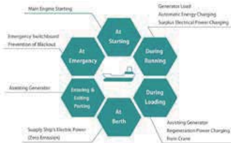
Fig.1 Applications of Li-ion Batteries on Ships
